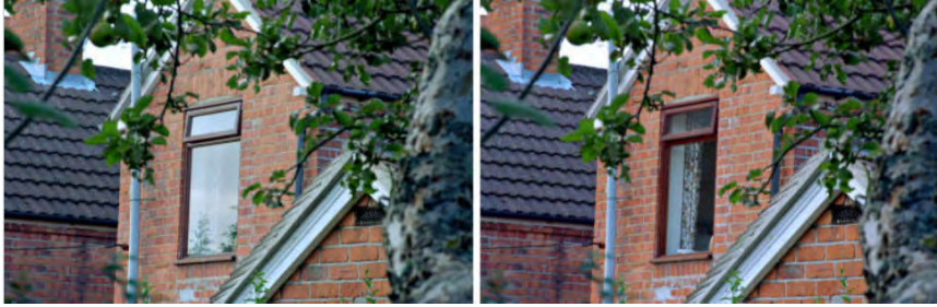
Figure 15.3: Because the TM and TE lights will be reflected differently, polarizer filter can produce remarkable effects on the quality of the photograph by reducing glare [97].
